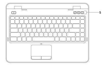
Windows Mobility Center button — Press to launch the Windows Mobility Center. Windows Mobility Center provides quick access to your mobile PC settings such as brightness control, volume control, battery status, wireless network and so on.
